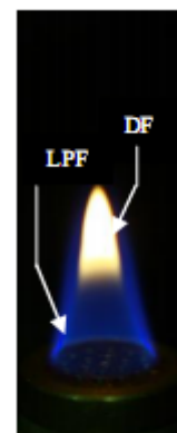
Fig. 9 Triple flame shape of KSO at \phi = 0.75
