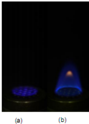
Fig. 3 view of KSO (a) perforated flame at \phi=0.44 , triple flame at \phi=0.62
