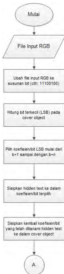
Gambar 8 Flowchart Proses Embed Metode LSB
